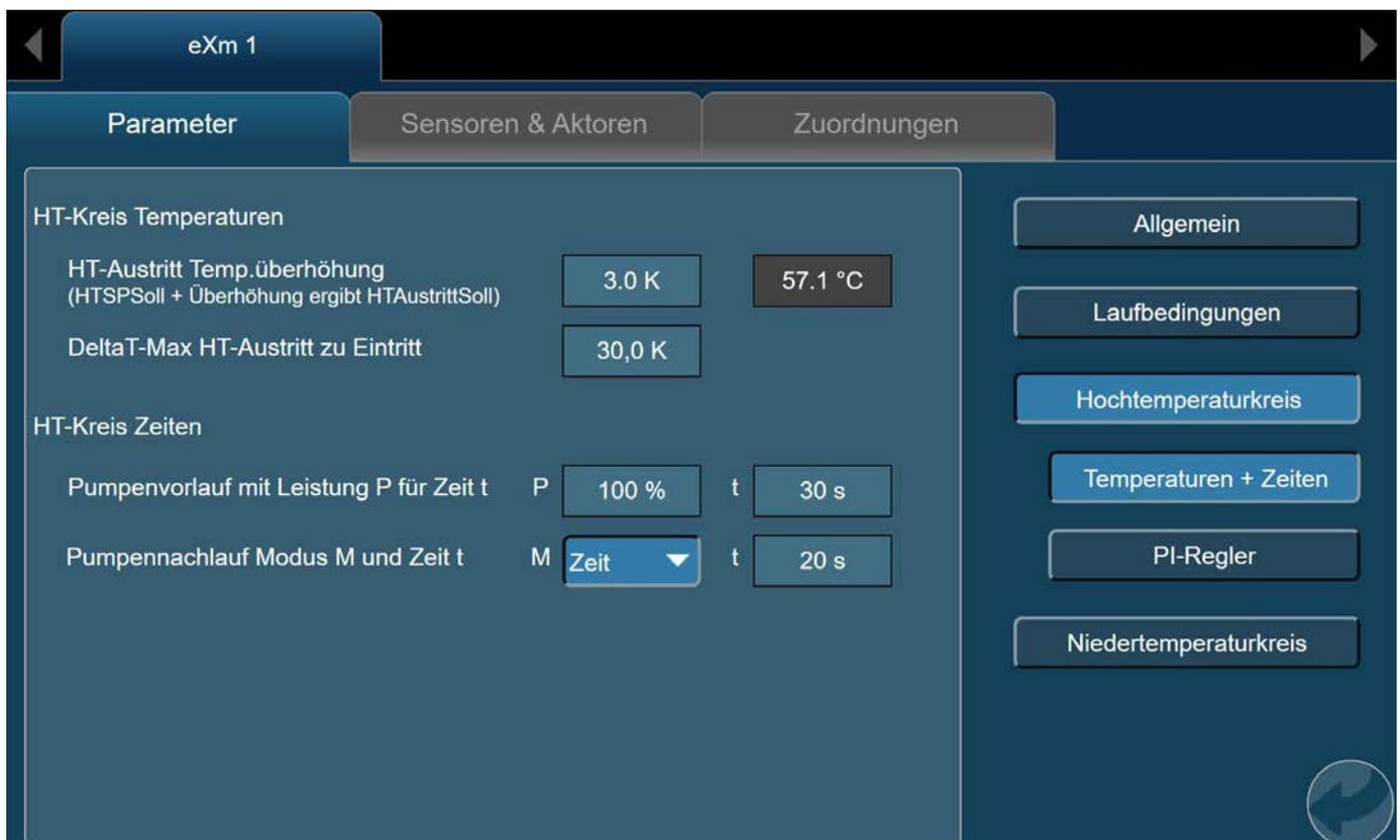
The screenshot shows the 'eXm 1' control interface with three tabs: 'Parameter', 'Sensoren & Aktoren', and 'Zuordnungen'. The 'Parameter' tab is active, displaying the following settings:
